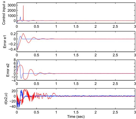
Fig. 4. Evolution of control input  $u$  and disturbance  $d$  for RHONN's (red line) and F-HONNF approach (blue line)
