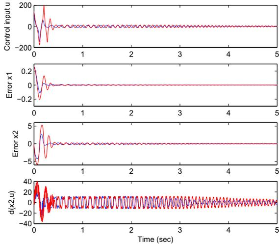
Fig. 2. Evolution of control input  $u$  and disturbance  $d$  for RHONN's (red line) and F-HONNF approach (blue line)
