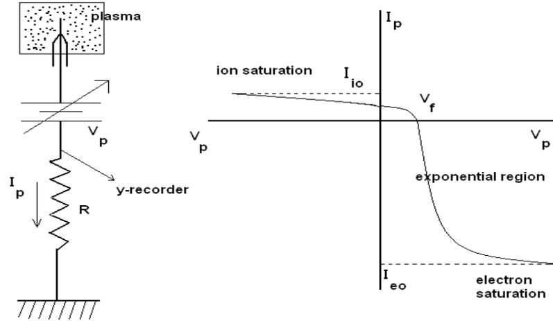
Figure 1. The Langmuir probe and its characteristic.
