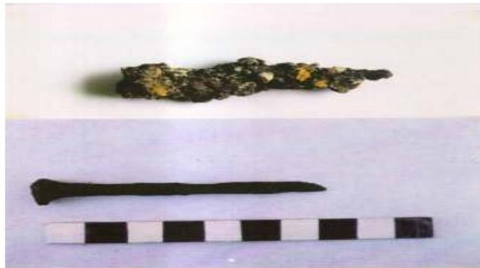
**Photo 1.** An excavated nail before and after plasma treatment.
