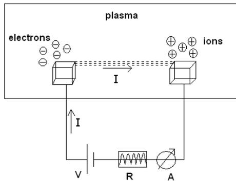
Figure 2. The external dc potential circuit during plasma treatment.
